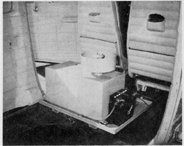
Fig. 2. Location of the oil injector in the cabin of the Desert Research Institute Cessna 206.
